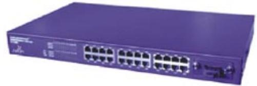
Ethernet switches are typically much more expensive than Hubs - their more passive cousins. Ethernet switches processors, memory, and firmware.
