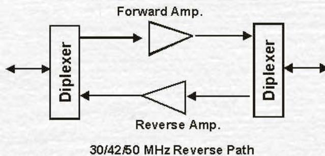
The few networks that utilised the reverse paths did so for relay of one channel. These users soon realised that the frequency band below 20 MHz was almost unusable due to the high amount of noise. This concern remains even today.
