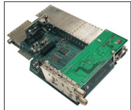
A transmodulator handles all channels on one satellite transponder and typically you will of course insert transmodulators where you obtain the maximum net increase in network capacity. If you are already distributing four channels from a selected transponder, digital compression "releases" 3 channels (3 x 8 MHz) in addition to distribution of all channels on the transponder.
