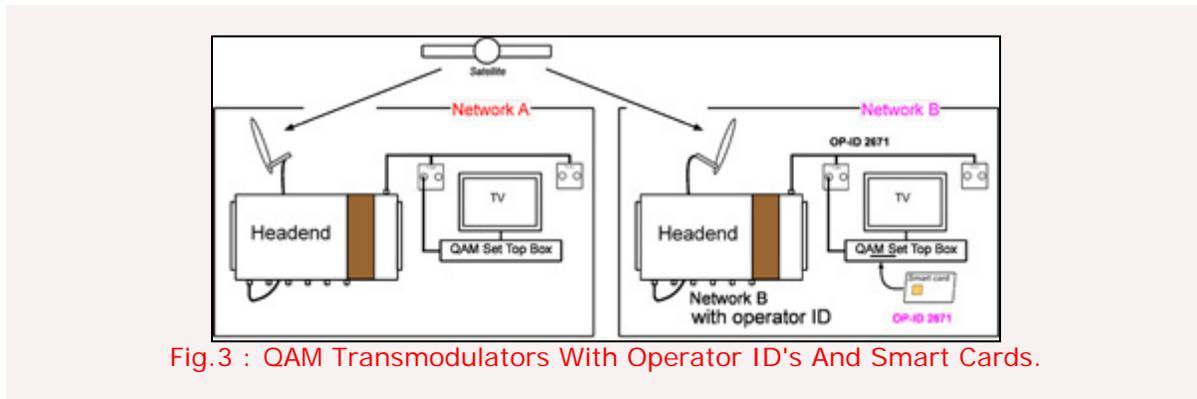
Fig.3 : QAM Transmodulators With Operator ID's And Smart Cards.
