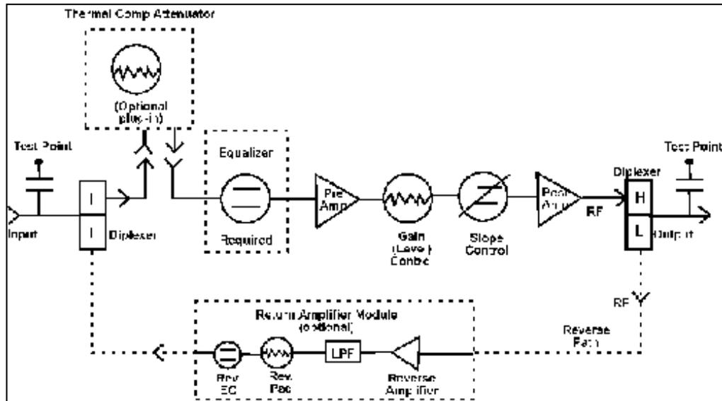
The signal partially amplified by the pre amplifier section now passes to the main gain and slope controls. As the name suggests, the gain control allows user setting of the output signal level. The slope control permits setting of the overall slope required
