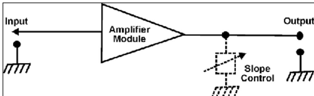
The line extender amplifier is a Hybrid IC based, single stage amplifier that offers reasonable performance at an attractive
