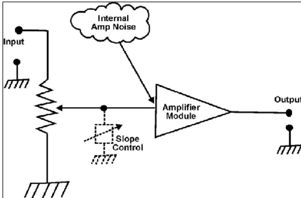
Figure 2 shows an alternate block diagram where the output signals are varied by the use of an attenuator across the output of the CATV Amplifier. This layout has the disadvantage that the amplifier module is constantly providing the highest output. Only a part of this output signal
