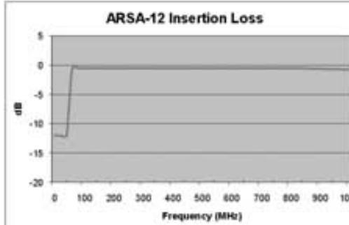
Return step attenuators (RSAs) provide much of the benefit of installing a high pass filter while retaining the ability for two-way operation. RSAs have minimum attenuation at frequencies used for the downstream (50 ñ 1000 MHz) and fixed attenuation at frequencies used for the upstream (5- 42 MHz). RSAs are available in attenuations that range from 3 to 25 dB.
