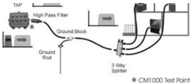
Simply removing the filter and installing a two way set top box or modem exposes the network to ingress the potential problem the filter was intended to eliminate in the first place.
