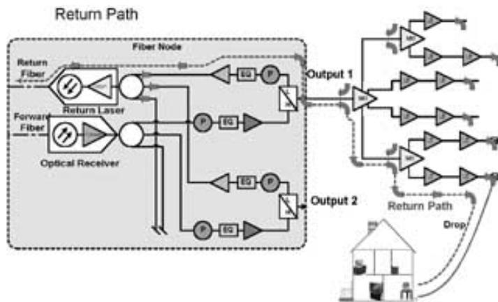
Studies indicate that most sources of ingress occur inside the home. It is therefore important that installation personnel use the proper techniques and are properly equipped so that two-way installations minimize pick up of ingress and noise. This will ensure reliable operation, fewer truck roles, lower maintenance costs and higher customer satisfaction.
